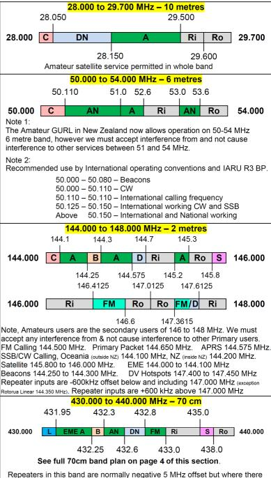
are problems with SRD/LIPD devices on the repeater input a suitable positive offset repeater frequency pair can be obtained from ELG. These frequencies are, or may be, allocated for use by other services. Amateur operators must accept interference from, and must not cause interference to, such other services. 433.05 - 434.79 MHz is also allocated for LIPDs, Industrial, Scientific and Medical (ISM) purposes.
