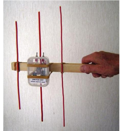
A Yagi antenna can be used for receiving and transmitting so the "driven element" can be either a diode receiver or a transmitter unit as shown in these two pictures.
