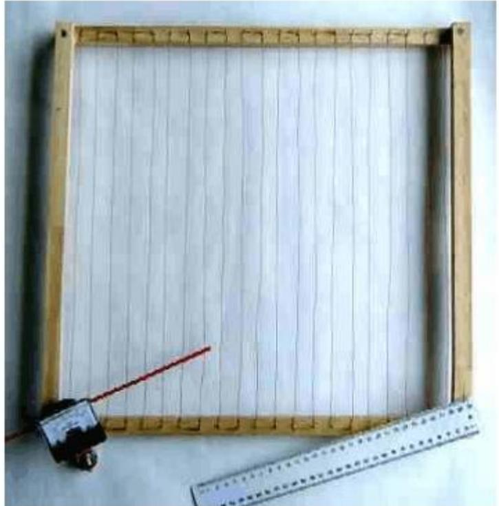
When the glue has set, small nails are tacked at 20 or 30 mm intervals along two opposite sides of the frame as shown in the photograph.
