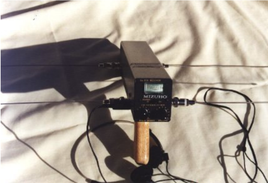
Figure 2 shows a Japanese ARDF receiver. This is an excellent commercial design packed full of features. The unit is available from Apex Communications. (1)
