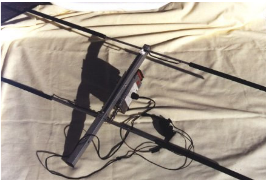
Figure 3 and 4 are a couple of views of Ron Graham VHF receiver. This is an AM dual conversion superhet' based on the MC6632 chip. It is tuneable over the bottom part of 2 metres and includes an audio signal strength indicator. The antenna is a modified HB9V.
