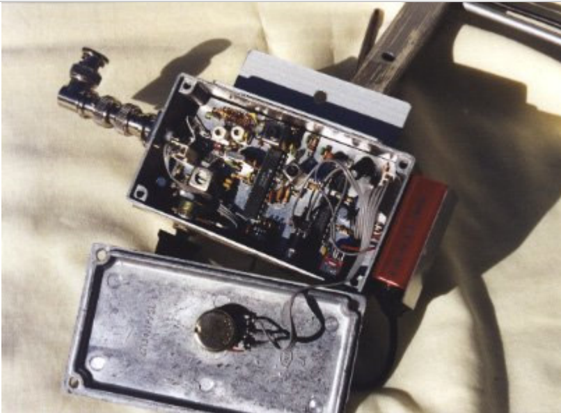
The Auckland VHF (3) group has available a microprocessor key that will meet most requirements. Figure 5. This was designed to interface with handhelds to provide clubs a quick and easy way to provide VHF ARDF transmitters, it also includes a output for key a 80 m transmitter.
